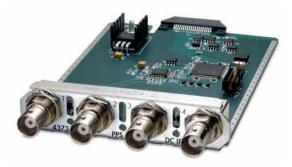
The 1PPS output card provides pulse outputs through four BNC connectors. These outputs are phase locked to the host receiver's disciplined reference oscillator. They are automatically enabled upon initialization and are independently selectable by the user with no configuration setup required.
