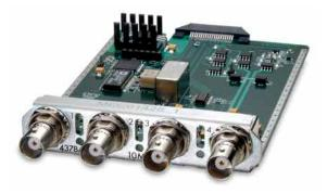
The 10MHz output card provides four low phase noise sine wave outputs through four BNC connectors. These outputs are phase locked to the host receiver's disciplined reference oscillator. They are automatically enabled upon initialization and are independently selectable by the user with no configuration setup required.
