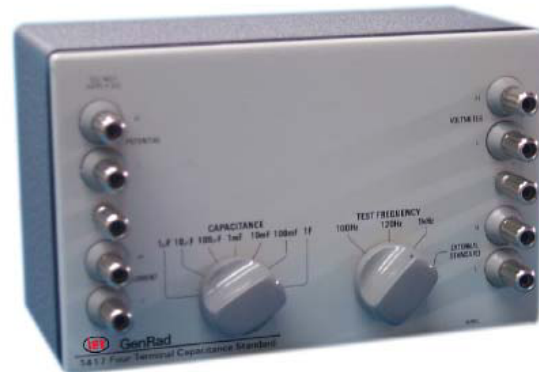
Model 1417 Capacitance Standard
