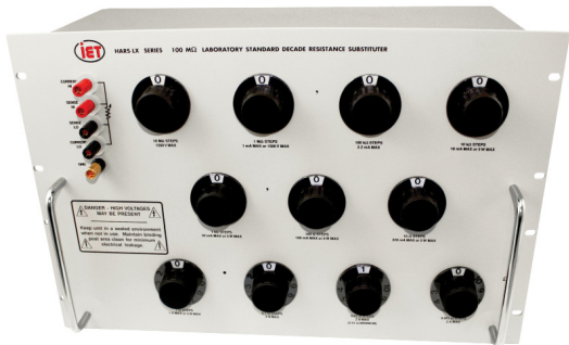
Eleven-decade model with 1 mΩ resolution, offering wide range and high resolution
