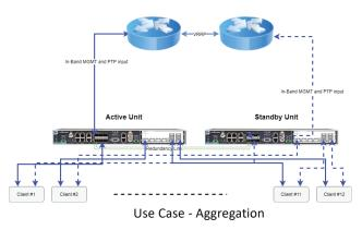
Accuracy is the relative offset between the active and standby units and is lower than 5 ns relative to the 1 PPS output on the active unit. A single IP management address is used. Health metrics and check mechanisms ensure proper monitoring of units to trigger the redundancy mechanism (switch over event). The redundancy schema is non-revertive. Manual intervention is required if the user decides to switch back to the original active unit once it is back in operation.
