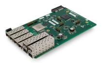
The 1 GbE/100 Mbps/10 GbE expansion module provides 1 GbE fanout and 10 GbE support. The module features four SFP and four SFP+ ports to enable a combination of four 100 Mbps Fast Ethernet and four 1 GbE ports, or eight 1 GbE ports, or a combination of four 1 GbE ports and four 10 GbE ports. As networks evolve, 10 GbE has become more prevalent, so this internal fanout capability is critical to connect to newer network elements.
